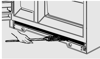
Clean the condenser coils at least once a year.
